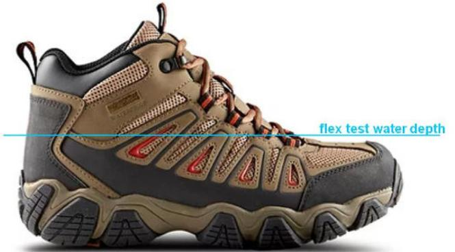
b) SATRA TM230: 2017 Dynamic water penetration, **up to** 100,000 flexes<sup>(1)</sup>, water just over vamp, mass gain included
